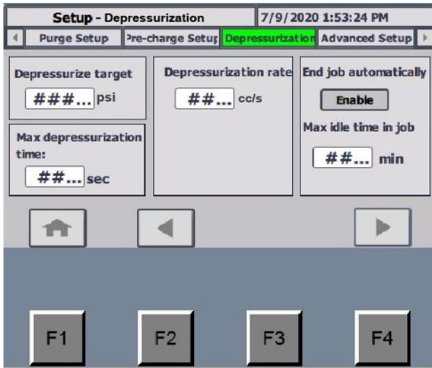
FIG. 25 De-pressurization Setup Screen
